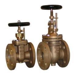
Non rising stem, metal seated gate valves. Suitable for cold and hot water, seawater, saturated steam, oil and other neutral non aggressive liquids.
