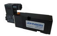
The JV231001 solenoid operated spool valve has threaded port connections and a NAMUR interface and can be easily adapted to a 3/2 function for controlling a spring-return single-acting actuator or to a 5/2 functions for controlling a double-acting actuator.
