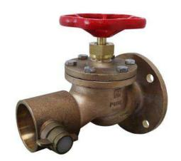
Marine grade bolted bonnet fire hydrant valve suitable for both offshore and onshore applications. Constructed with a dual seat design, the primary valve seat is NBR with an additional secondary metal to metal seat.
