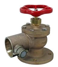
Marine grade bolted bonnet fire hydrant valve suitable for both offshore and onshore applications. Constructed with a dual seat design, the primary valve seat is NBR with an additional secondary metal to metal seat.
