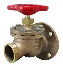
Marine grade bolted bonnet fire hydrant valve suitable for both offshore and onshore applications. Constructed with a dual seat design, the primary valve seat is NBR with an additional secondary metal to metal seat.
