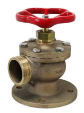
Marine grade bolted bonnet fire hydrant valve suitable for both offshore and onshore applications. Constructed with a dual seat design, the primary valve seat is NBR with an additional secondary metal to metal seat.
