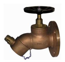
This bib nosed pattern fire hydrant valve with screwed bonnet is suitable for both offshore and onshore applications. Constructed with a dual seat design, the primary valve seat is hard rubber with an additional secondary metal to metal seat.
