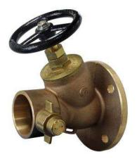
This straight pattern fire hydrant valve with screwed bonnet is suitable for both offshore and onshore applications. Constructed with a dual seat design, the primary valve seat is hard rubber with an additional secondary metal to metal seat.
