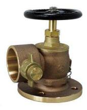
This angled pattern fire hydrant valve with screwed bonnet is suitable for both offshore and onshore applications. Constructed with a dual seat design, the primary valve seat is hard rubber with an additional secondary metal to metal seat.
