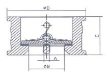
JV081016 Cast Iron (Epoxy Coated) Body EPDM Seat Dual Plate Spring-Loaded Check (Non-Return) Valve Length A Multi-Flange Wafer Type PN10/16 & ANSI 150
