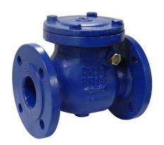
A robust ductile iron, swing type (flapper) check valve with a ductile iron disc and bronze trim suitable for cold and hot water, seawater, fuel oil and other non-aggressive medium.
