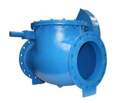
The JV080037 is a metal seated swing check (non-return) valve with EPDM seals used to prevent reverse flow. In this case an outside lever and weight is fitted to the standard valve to aid closure when gravity is insufficient to close the valve fast enough.
