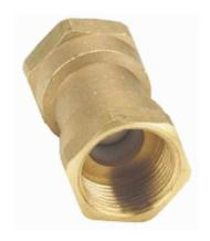
A WRAS approved economical spring-loaded non-return valve with a DZR brass body and EPDM seals. The valve requires a minimum pressure of 0.1 bar to open and can be installed in both horizontal and vertical lines with upward flow or in any intermediate position.
