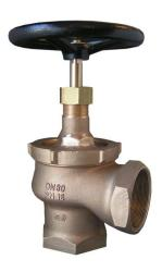
These robustly constructed bronze, secured union bonnet globe valves are ideally suited for sea water and low pressure steam isolation applications in area's on board ships where a light bronze construction is desirable. These valves can also be supplied with an optional regulating disc.
