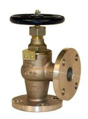
Bronze metal seated gland packed globe valve to JIS Japanese specifications. Suitable for cold and hot water, seawater, saturated steam, oil and other neutral non aggressive liquids.
