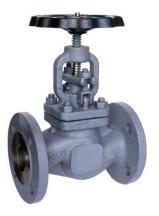
This bolted bonnet globe valve with a stainless steel valve disc is ideally suited for isolation duty, providing a leak tight shut off with the capability of being used partially open to regulate flow.
