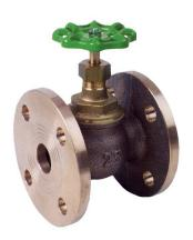
An economical bronze globe valve with a PTFE valve disc with a non-return design, preventing reverse flow when in the open position. Also suitable for isolation duty, providing a leak tight shut off.
